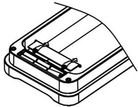
2. Install the batteries into battery box, please mind the polarity (6xAA – not included)
