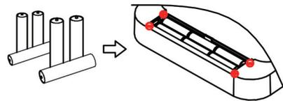
3. Push battery cover to close position, make sure the clip snap firmly
